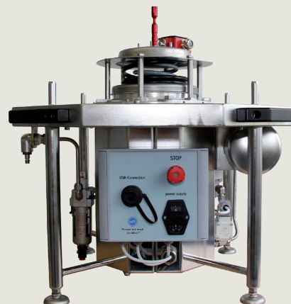
MESSKO® MPREC test bench with installed pressure relief device
